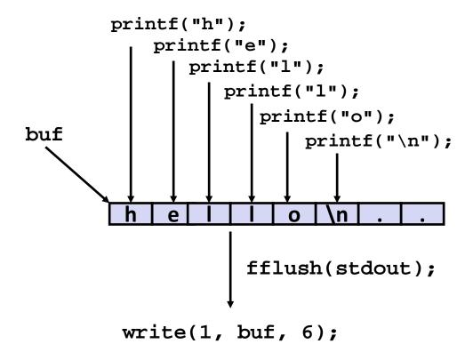
Buffer flushed to output fd on "\n", call to fflush or exit, or return from main.
