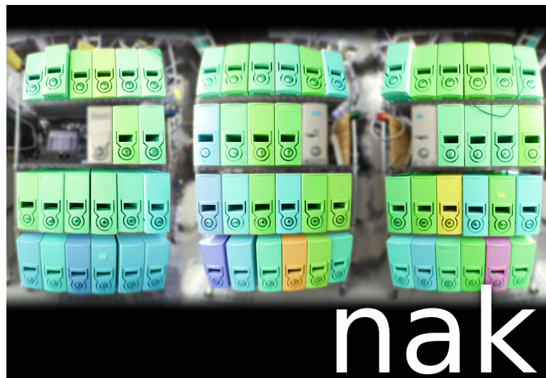
Figure 2.1: A temperature display from NodeScape v1
