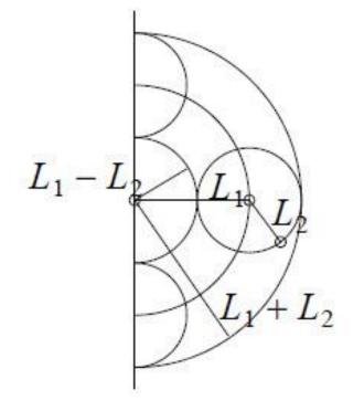
Underconstrained system: relatively few constraints on the configuration and there are many solutions to the problem posed
