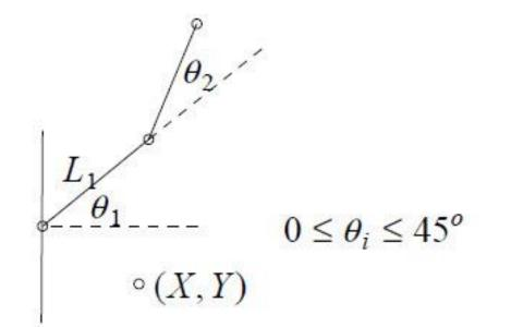
Underconstrained system: relatively few constraints on the configuration and there are many solutions to the problem posed
