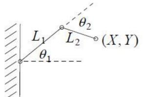
Given the desired position (*X*, *Y*) for the end effector  $(L_1 - L_2 \le \sqrt{X^2 + Y^2} \le L_1 + L_2)$  find joint angles  $\theta_1$  and  $\theta_2$  so that the corresponding position of the end effector is (*X*, *Y*). Analysis:
