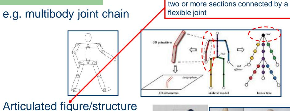
Articulation: movement of an **appendage** by changing the configuration of a joint
