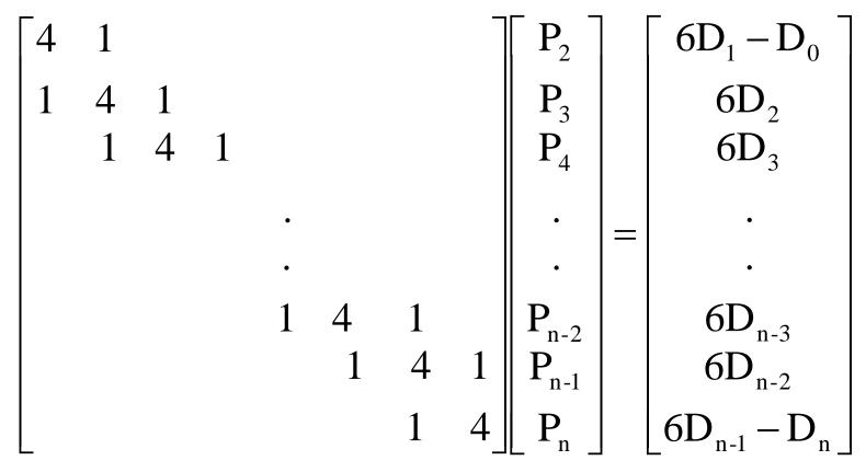
**This system of equations can be solved using 2Gaussian elimination without pivoting.** CS Dept, UK
