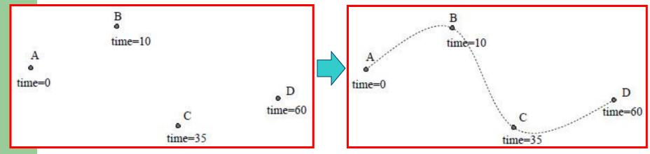
• Want: a curve interpolating these position-time pairs
