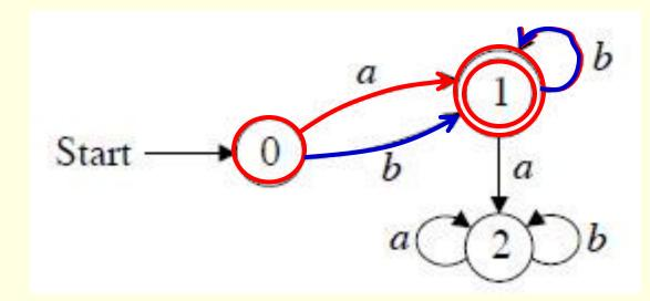
**Example.** The example DFA accepts the strings *a, b, ab, bb, abb, bbb, ..., ab<sup>n</sup>, bb<sup>n</sup>, ...*
