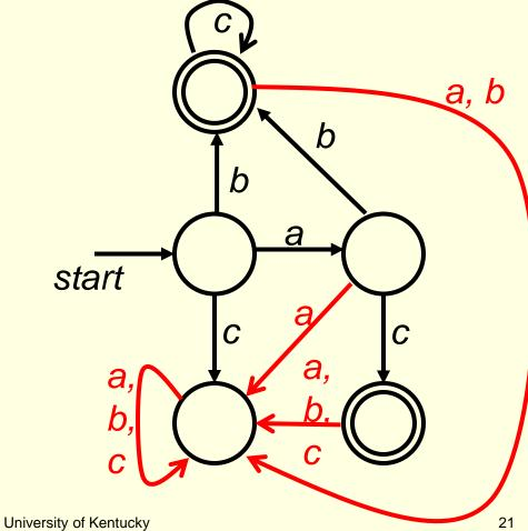
To make each of these FA's a DFA, you either create a new state or use a non-final state as the sink of all the remaining edges of the FA, or both.
