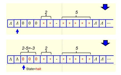
Your task here is to fill out the six blanks in the following figure to make it a TM that can subtract a bigger number from a smaller number as well.
