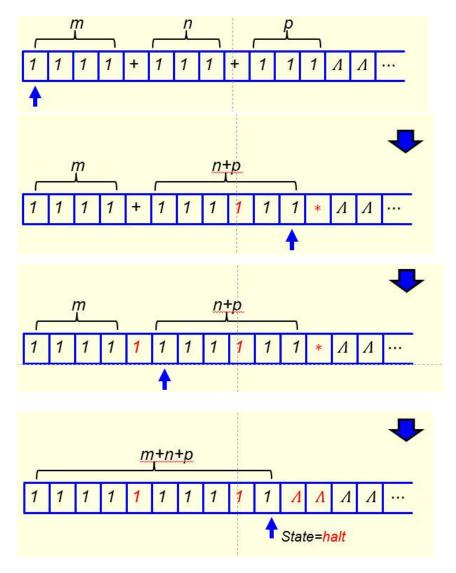
Your task here is to fill out the five blanks in the following figure to make it a TM that can perform addition on three given non-zero positive numbers in unary form directly.
