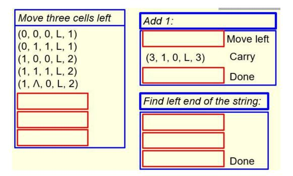
and then fill out the blanks in the following chart to make it a complete state transition diagram for this TM. Make sure the instructions you choose fit into the diagram naturally and logically. In the diagram, state H means the 'Halt' state. You have to use your own text boxes here too. (1 point each blank)
