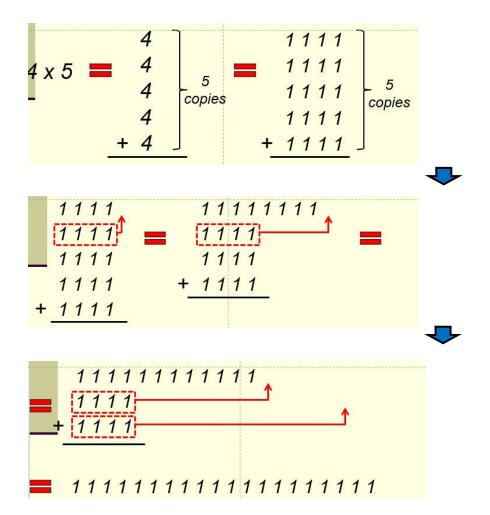
Your task here is to fill out the three blanks in the following TM that does multiplication of two given numbers m and n in unary form. Note that the portion circled by the red dotted curve is to perform the addition job (putting a copy of m 1's at the end of n) and the portion circled by the blue dotted curve is the portion that does the counting (making sure n copies of
