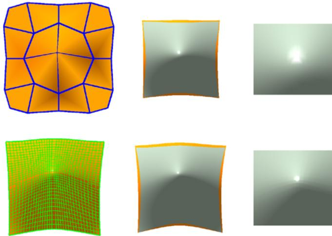
Fig. 9: Comparison of offsetting surface after 3 recursive subdivisions on CCS mesh: (a) CCS control mesh, (b) generated offsetting surface, (c) enlarged central part of the offsetting surface.
