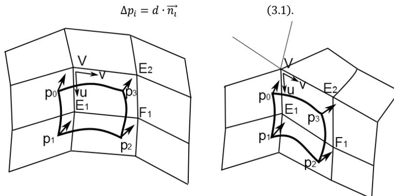
Fig. 6: CCS control mesh and its corner data points and normals: (a) regular face, (b) extraordinary face
