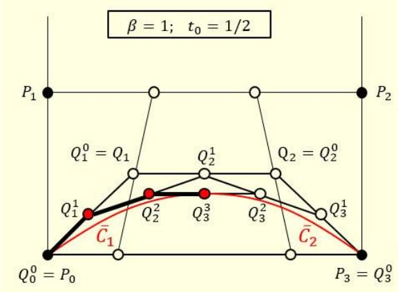
Figure 11. Subdivision of a cubic Beta-Bezier curve segment with shape parameter  $\beta = 1$  at  $t_0 = 1/2$ .
