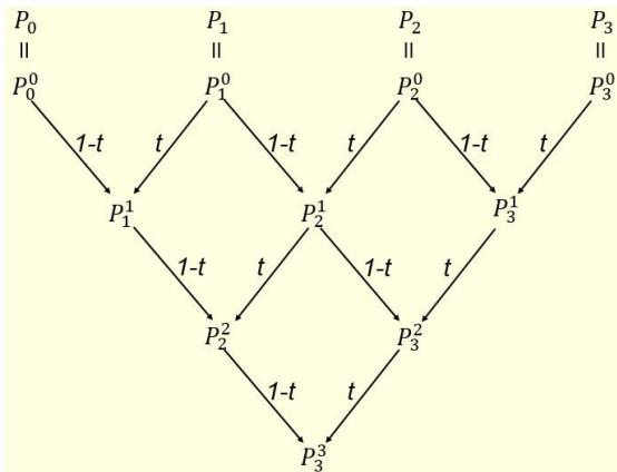
Figure 6. Computation flow of the de Casteljau algorithm for a cubic Bezier curve.
