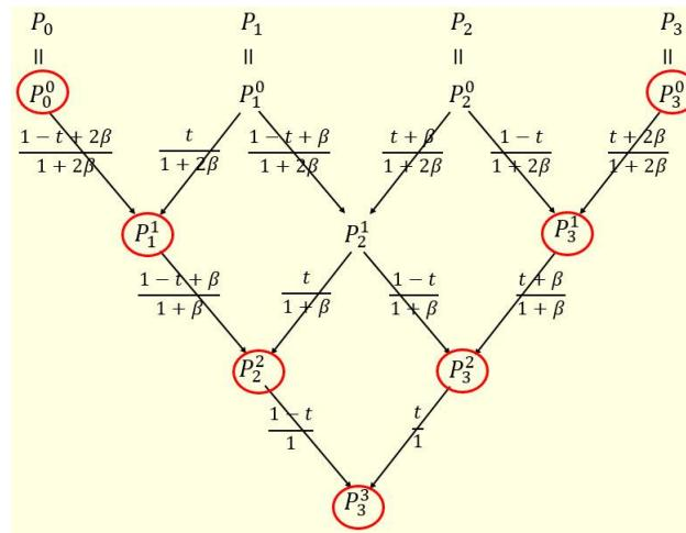
Figure 8. Computation flow of the de Casteljau algorithm for a cubic Beta-Bezier curve.
