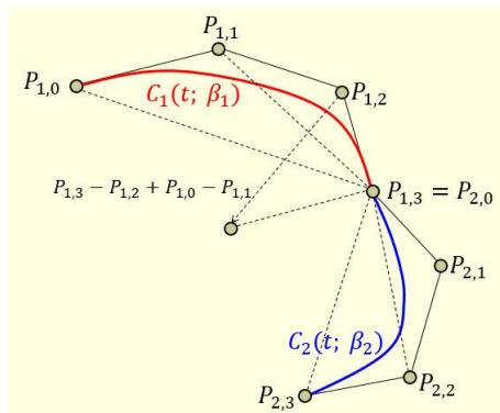
Figure 9. Connecting two cubic Beta-Bezier curve segments.
