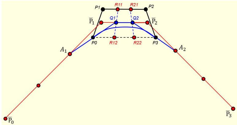
Figure 13. Representing a cubic Beta-Bezier curve segment as a cubic B-spline curve segment.
