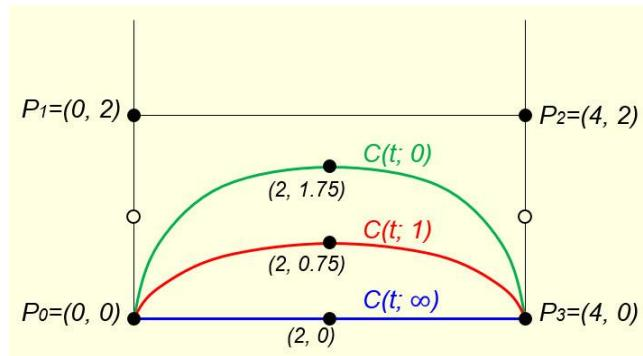
Figure 3. Cubic Beta-Bezier curves defined by the same control points but with different shape parameters.
