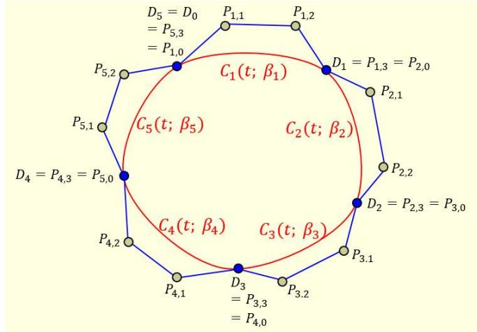
Figure 12. Interpolation using a composite cubic Beta-Bezier curve.
