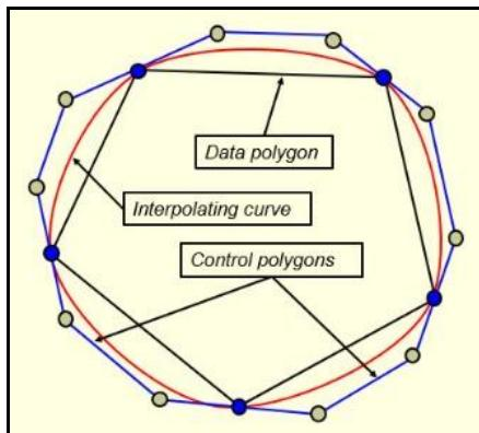
Figure 2. A composite cubic Bezier curve that interpolates a set of data points.
