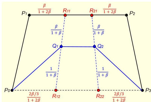
Figure 4. Relationship between control points of a cubic Beta-Bezier curve and its Bezier control points.
