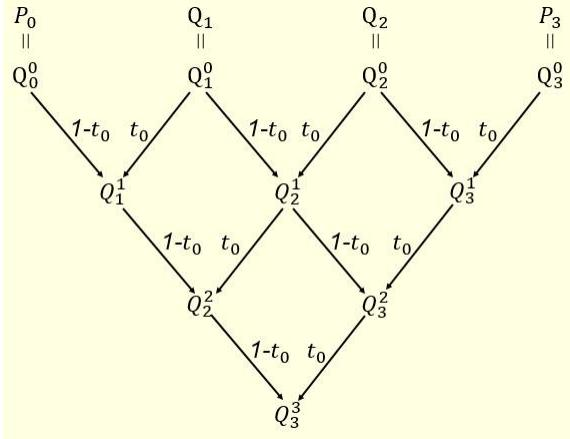
Figure 10. Computing the value of  $C(t; \beta)$  at  $t_0$  when represented as a cubic Bezier curve.
