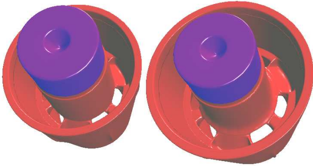
Figure 9: Constrained scaling of a marker cap: before scaling (left), after scaling (right) with S_x = 1.2 , S_y = 1.2 S_z = 1.0 .
