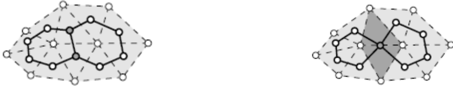
Figure 4: Illustration of edge contraction in dual graph (defined by solid edges) [19]. Left: dual graph before edge contraction; Right: dual graph after edge contraction, where two nodes in shaded area are merged into a single node.
